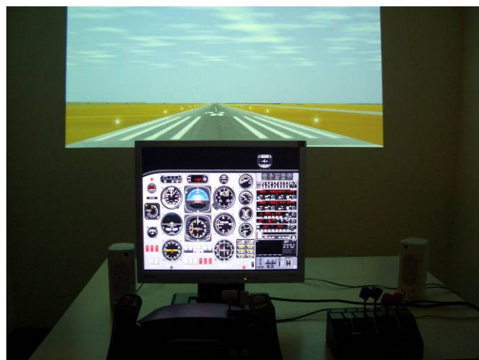
Figure 1: Elite Version 8.0 basic flight training device.
